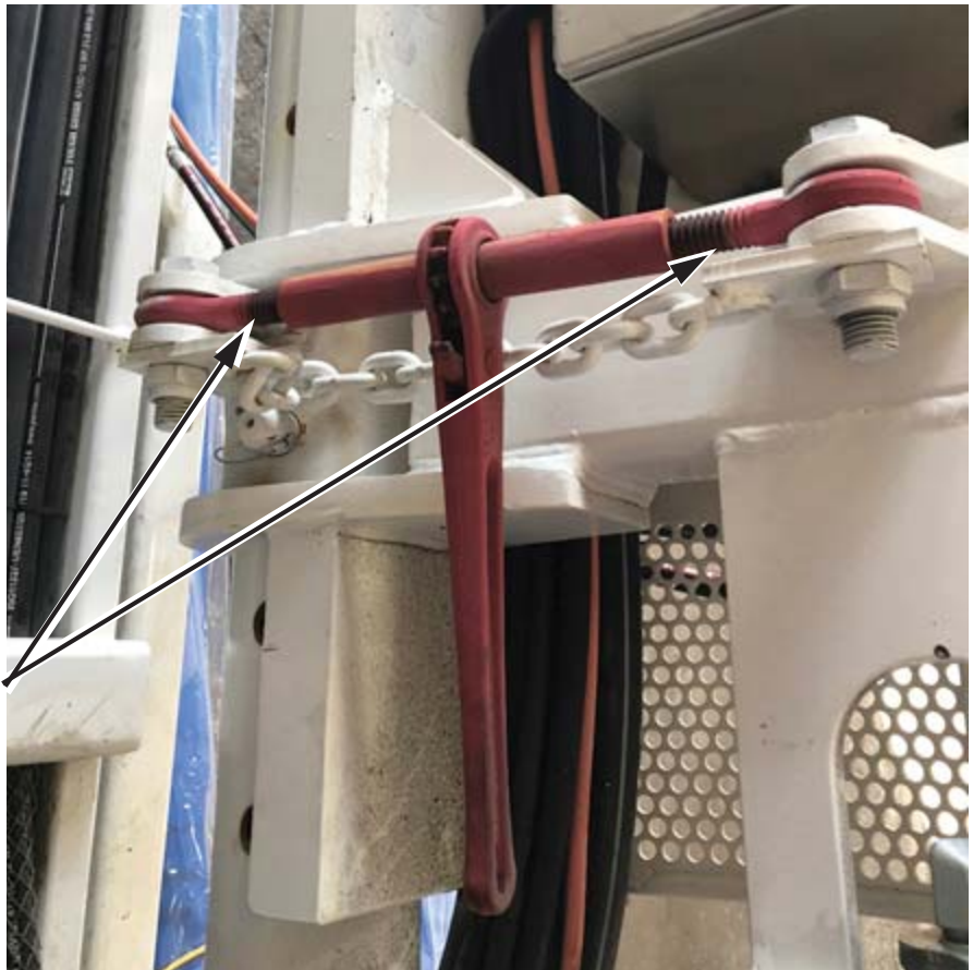
Figure 1: Load Binder shown in center position without safety securement
