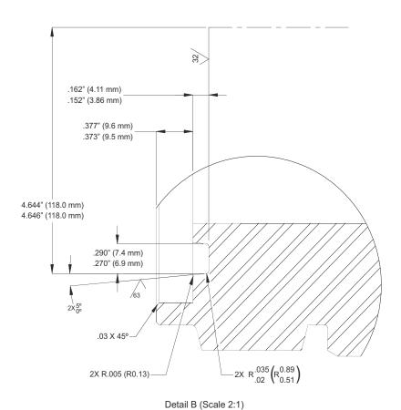
Figure 2: Upper Quill with New Counterbore Feature for Washout Plate
