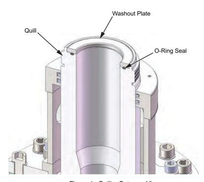
Figure 1: Quill - Cutaway View
