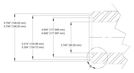
275, 350, & 500 Ton Quill Modification Section View of Washpipe Retaining Area
